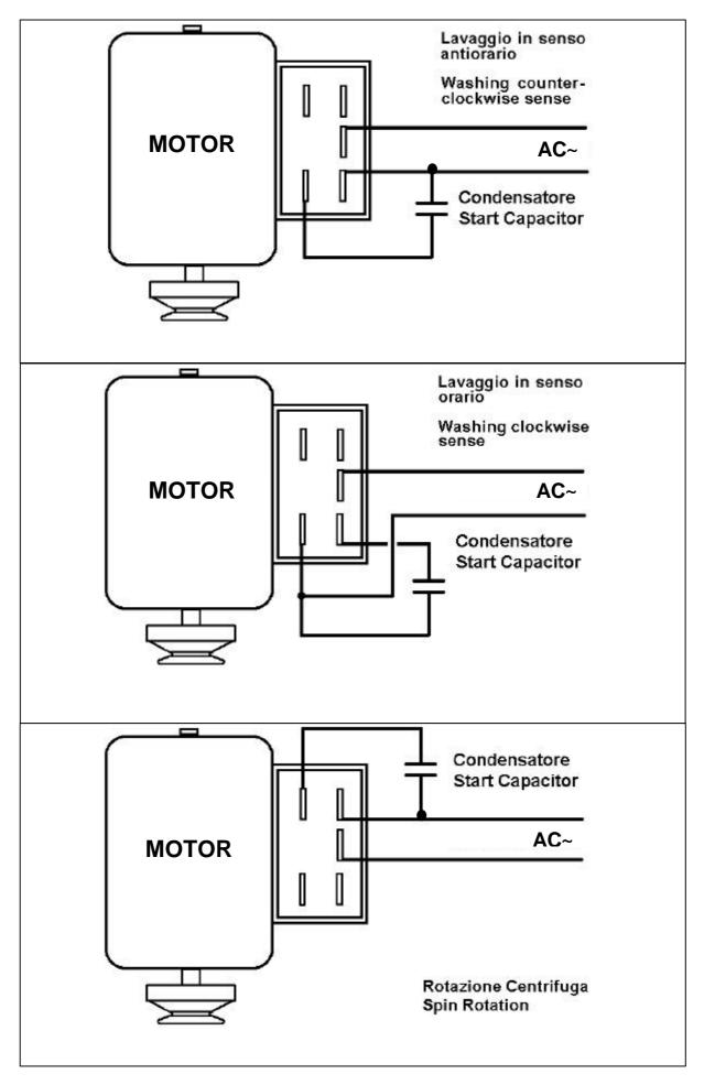
A2) Induction motors with "B" type connector (Common Contact Internal).
