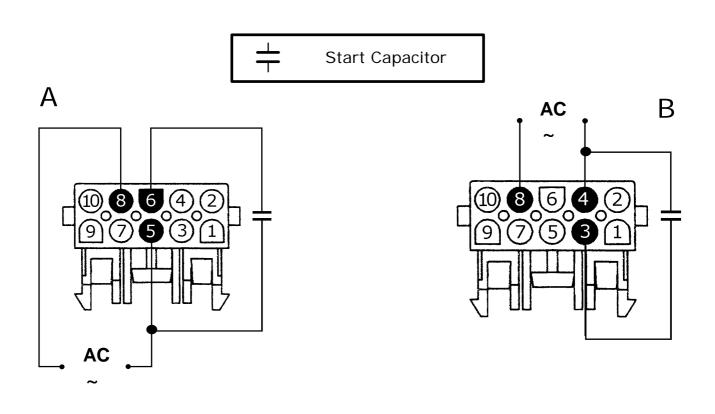
A = Testing <u>counterclockwise</u> spin rotation. B = Testing <u>clockwise</u> rotation during washing.
