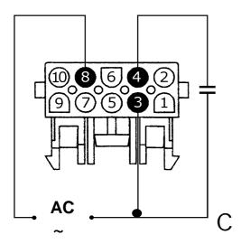
C = Testing <u>counterlockwise</u> rotation during washing.
